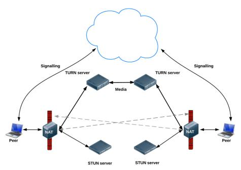
Figure 2.1: WebRTC Signalling
